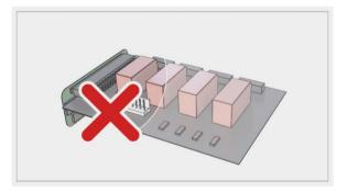
① Raspberry Pi Zero should be connected pointing upwards, not downwards
