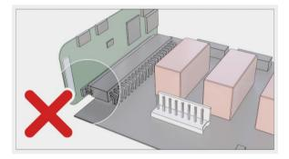
1 Make sure pins are properly aligned when connecting
